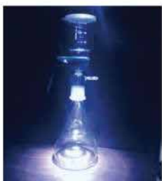
5350 - All Glass Filter Holder - 47mm, Filtration Assembly
